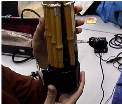
Figure.4 the air-pressure sensor for SHO
