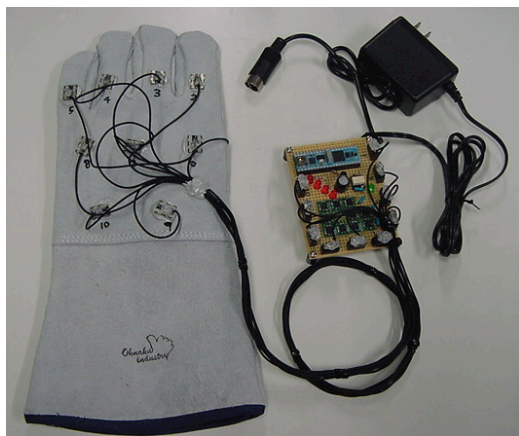
図10 "VFB10"の全景 Figure 10 The system "VFB10".
