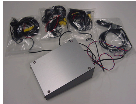
Fig. 2 Main sensor box and cables.
