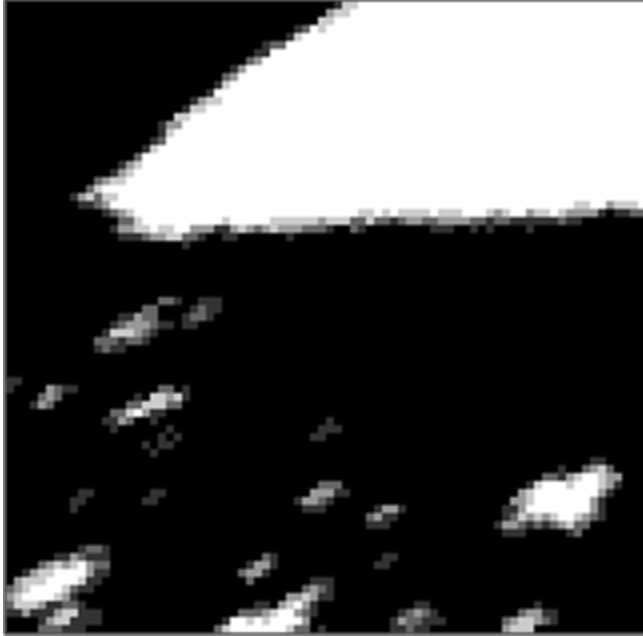
Figure 7. Five day composite of inland water mask in MOD10A1. The inland water mask, bit 0 of NDSI_Snow_Cover_Algorithm_Flags_QA was extracted for 7-11 January 2003 and composited. In this composite image of the southern end of Lower Red Lake in MN, black is land on all five days and white is lake on all five days, shades of gray are where the cell was not lake on all five days. Shades of gray from light to dark show where lake was mapped to the cell on from 4 to 1 days in the period. Shades of gray represent the geolocation wobble of lakes.
