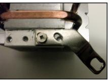
Repeat for the other 3 arms. Leave the screws a little loose, so the arms can wiggle a little bit. You'll tighten these in a few steps. Throw the other fan parts away, except for the thermal paste.
