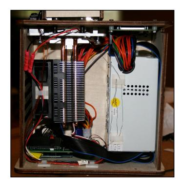
If the Power Supply wires are blocking the power supply fan, make sure to push them out of the way. The same applies to any other wires that might block OpenPCR's airflow.
