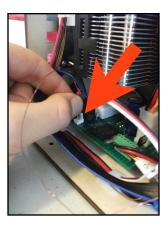
Wrap the heat block temperature sensor once around the clips on the power supply.
