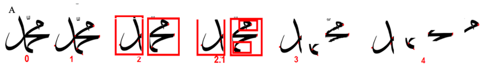
Figure 3 Steps of zone segmentation-based windows segmentation approach. 0, original image; 1, detection of junction and end points; 2, sliding window; 2.1, detection of ligature (applying algorithms 1 and 2); 3, application of algorithm (baseline detection for splitting the image into upper, middle, and lower zones); 4, segments resulting from baseline detection.
