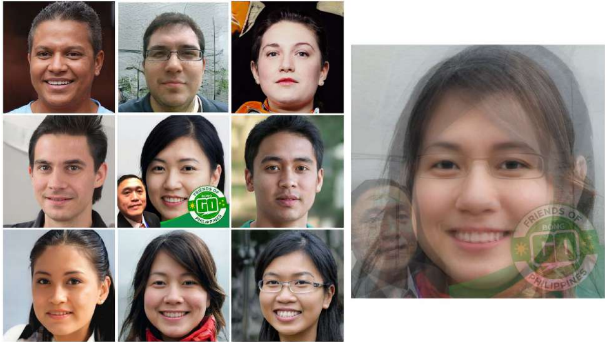
Left, nine profile pictures from the operation, some of which were cropped or had stickers added. Right, all nine images rendered opaque and superimposed to show the alignment of the eyes, an indicator of synthetic image generation.
