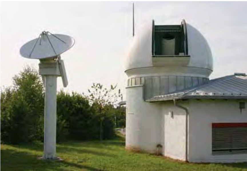
Figure 6.36. The Laser Ranging System of the geodetic observatory in Wettzell, Bavaria. (ILRS)
