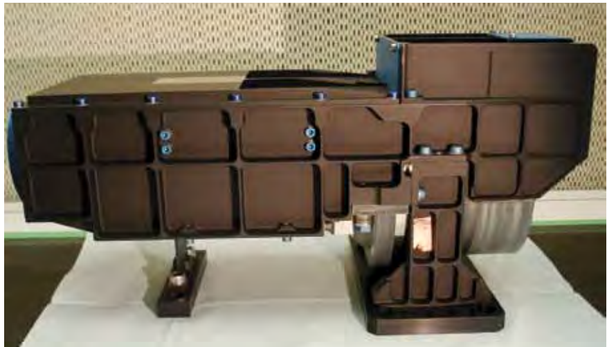
Figure 6.14. Engineering Model of one of five cameras of the Ocean and Land Colour Instrument. (TAS-F)
