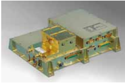
Figure 6.29. The GPS receiver unit. (TAS-F)
