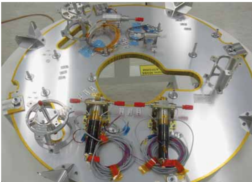
Figure 5.22. Integration of the latch valve into the propulsion panel. (TAS-I)
