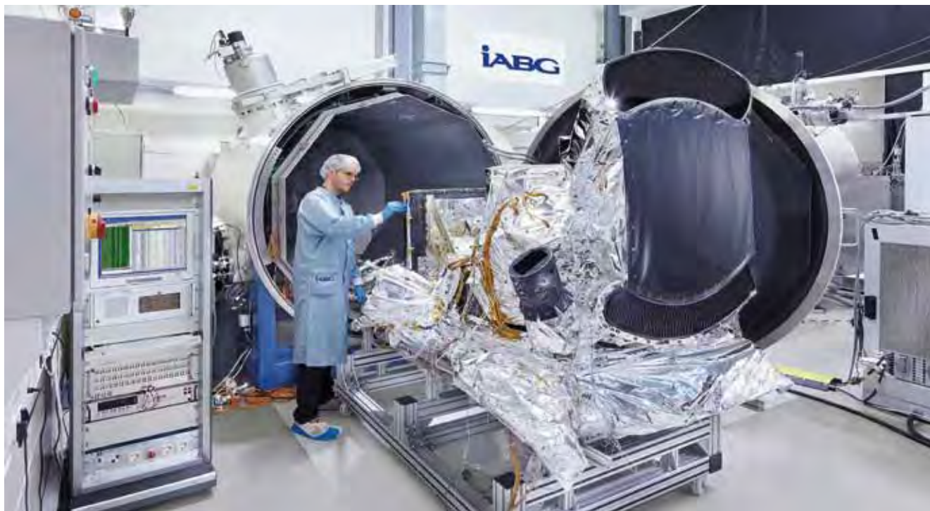
Figure 6.3. The SLSTR Optical Scanning Unit. (IASG)
