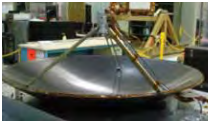
Figure 6.22. Engineering model of the SRAL antenna. (MDA)
