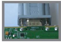
For Linux or Android development, connect the supplied serial cable to the UART-1/2 DB-9 connector. For WindowsCE development, connect to UART-3. Connect the other end of the cable to a PC or workstation.
