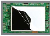
Remove the protective plastic from the LCD touchscreen.
