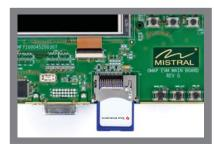
Choose the OS and insert the SD card into the AM/DM37x EVM as shown.
