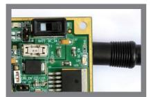
Connect the power cable to the power jack on the main board. It is recommended to complete this step before connecting the power source. As there is no power switch on the EVM, use the cord for power cycling the board.
