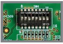
Ensure SW4 DIP switch is set as shown. SW4 DIP is located on the front of the AM/DM37x EVM main board.
