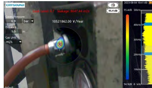
Camera-based air leak inspection
