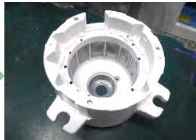
Wound coil component after BMC shaping
