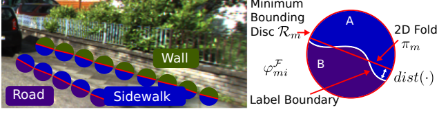
Figure 4: Geometric Unary Potentials. Left: We encourage label changes at 3D curbs or folds after projection into the image domain. Right: This constraint ( \varphi_{m_i}^F ) is implemented by pixel unary potentials inside each minimum bounding disc \mathcal{R}_m around each 2D curb or fold segment m .
