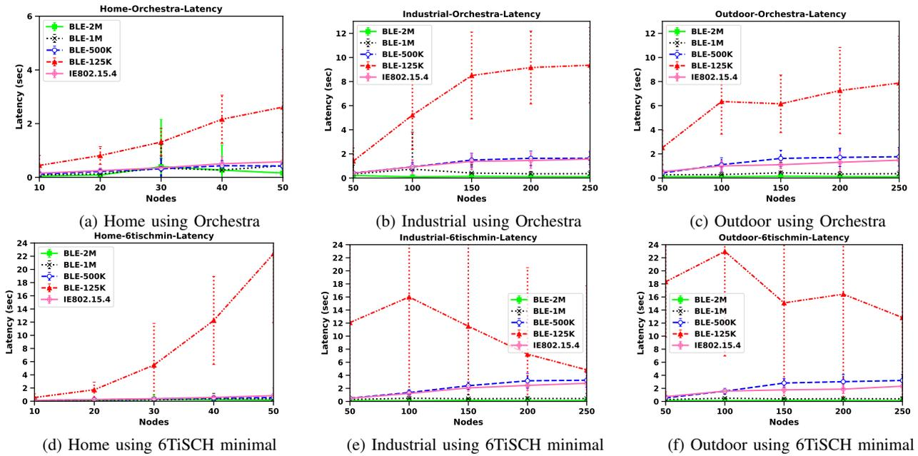
Fig. 2: End-to-end latency in seconds.
