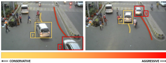
Fig. 4: GraphRQI Performance: GraphRQI classifies road-agent 1 (red bounding box) as threatening and road-agent 2 (yellow bounding box) as conservative. We plot the vector, w = \mathcal{L}u , where u is the eigenvector corresponding to the largest eigenvalue of \mathcal{L} , as a gradient below the figure.
