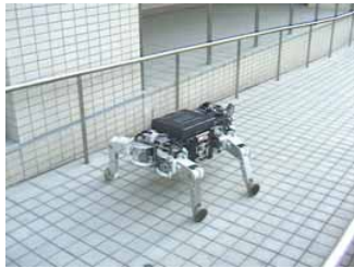
Fig. 6. Achievement of slope climbing propulsion ( \theta_0 = 0.4rad, \omega = 2.88rad/s, V = 0.32m/s )
