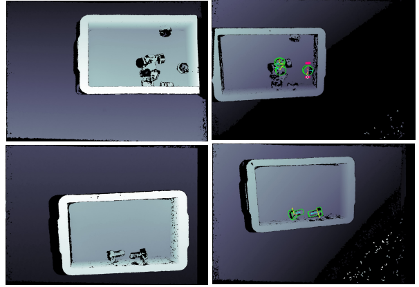
Fig. 12. The result of baseline B (random sensing + multi-view) versus ours. Objects in green represent successful 6D pose estimation. Left column: result of B; Right column: ours. Top row (mirror_nut) and Bottom row (small screw) are two different types of objects. Ours always observes the objects with proven recognition success in the last cycle and from the view center for better sensing results.
