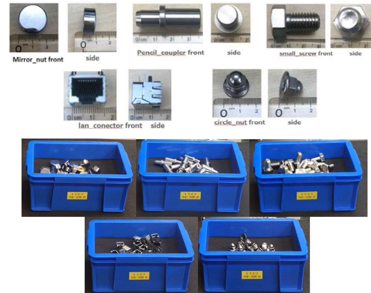
Fig 10 . Top: the 5 different target objects with shiny surfaces and different shapes. Bottom: 20 piled target objects in each box ( 50\text{cm} \times 25\text{cm} ) for picking experiments.
