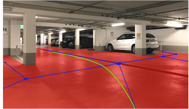
Fig. 1. Schematic illustration of the approximated free-space (red) and the roadgraph with direction options (blue). Based on the directional choice to go straight, a smooth path can be planned (green).
