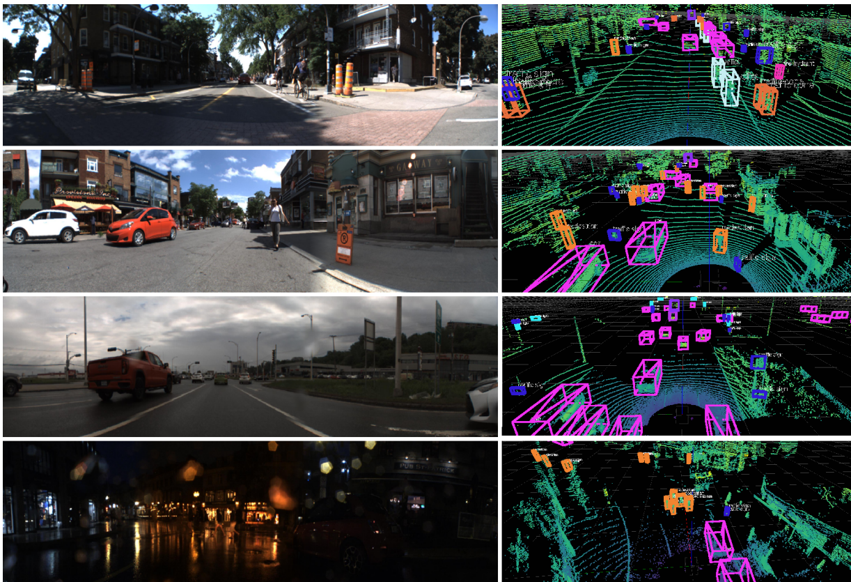
FIG. 7: PixSet dataset overview of the variety of scenes and environmental conditions with samples from the cameras and the OS1-64 LiDAR with 3D boxes annotation.
