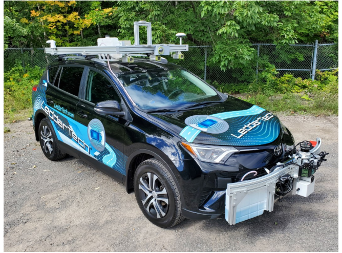
FIG. 1: Instrumented vehicle ( RAV4 ) used for data acquisition.
