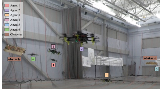
Fig. 1. Hardware demonstration of RMADER with 6 UAVs and 2 dynamic obstacles (UAVs shrouded with brick-pattern foam). Agents communicate over a mesh network that exhibits an average delay of 49.8 ms (483 ms max). Despite these communication delays, RMADER enables decentralized, asynchronous onboard planning resulting in UAVs flying with a maximum speed of 5.8 m/s.
