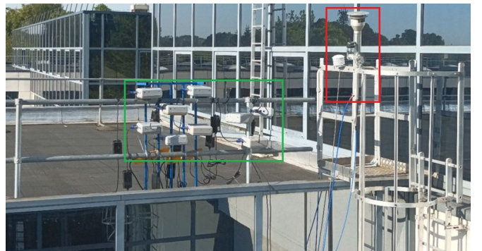
Figure 1: The experimental setup containing the 12 sensors (framed by green) and reference instrument measurement (sampling \text{PM}_{2.5} framed by red).
