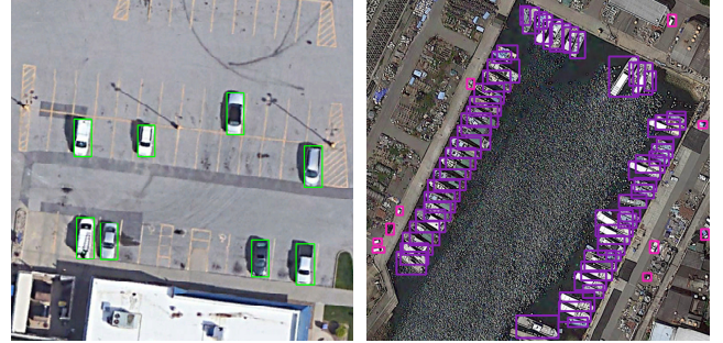
Fig. 1. Visualization of samples drawn from DIOR and DOTA. Here we can see that the distribution of objects in remote sensing images are globally sparse and locally dense.
