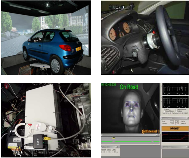
Fig. 5. SHERPA simulator (upper left). Steering system (upper right). Data acquisition system (bottom left). Continental driver monitoring system (bottom right).
