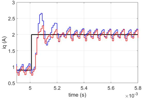
Fig. 15.  $i_q$  step from 0.9 to 3 A at  $\omega_m$  of  $50 \frac{rad}{s}$ . Reference current  $i_q$  (black line), FPGA DB  $i_q$  (blue line), OS-DB  $i_q$  (red line).
