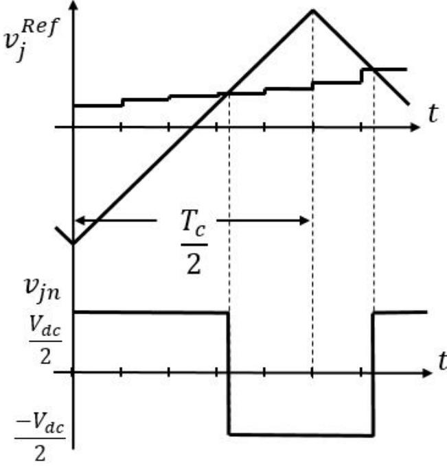
Fig. 2. PWM and phase leg voltage.
