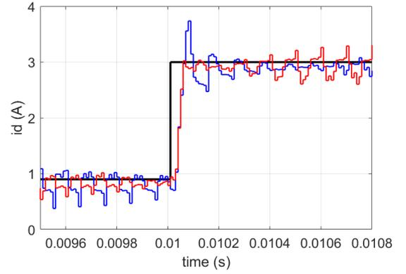
Fig. 13.  $i_d$  step from 0.9 to 3 A at  $\omega_m$  of  $100 \frac{rad}{s}$ . Reference current  $i_d$  (black line), FPGA DB  $i_d$  (blue line), OS-DB  $i_d$  (red line).
