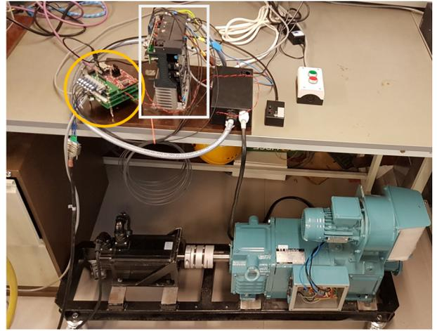
Fig. 9. Experimental set-up: 2L-VSI (white rectangle), control board (yellow circle) and motors.
