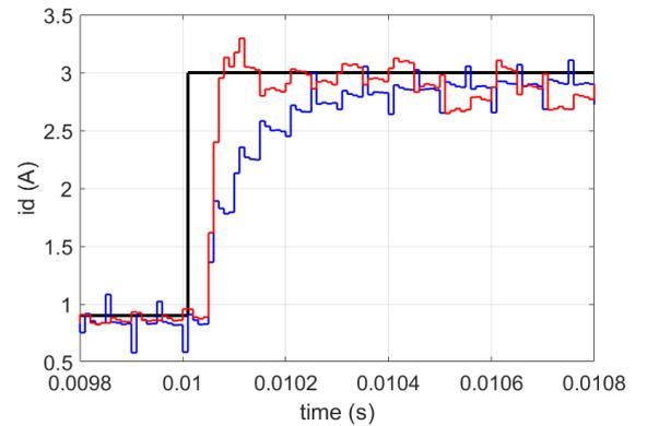
Fig. 14.  $i_d$  step from 0.9 to 3 A at  $\omega_m$  of  $50 \frac{rad}{s}$ . Reference current  $i_d$  (black line), FPGA DB  $i_d$  (blue line), OS-DB  $i_d$  (red line).
