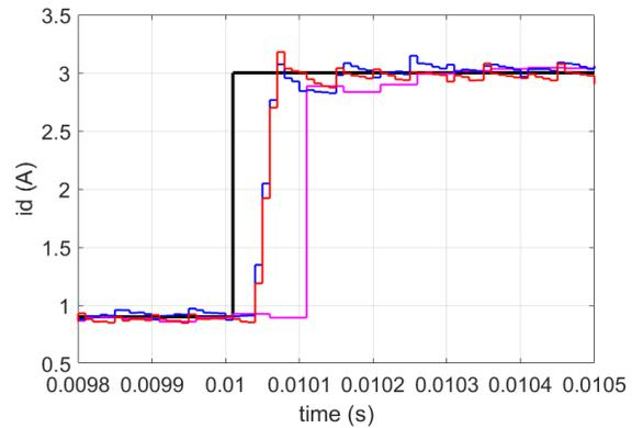
Fig. 10. System response to a reference  $i_d$  step from 0.9 to 3 A at standstill. Reference current  $i_d$  (black line), DSP DB  $i_d$  (magenta line), FPGA DB  $i_d$  (blue line), OS-DB  $i_d$  (red line).
