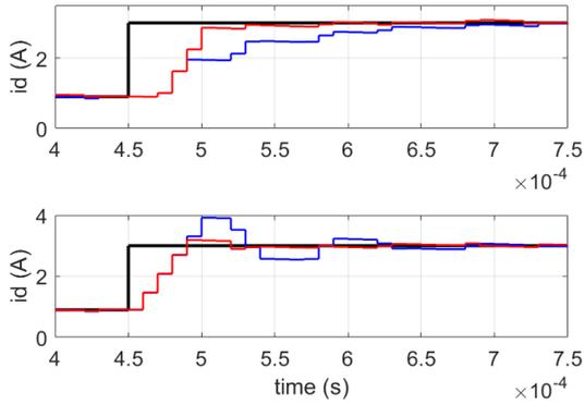
Fig. 7. OS-DB  $i_d$  step from 0.9 to 3 A at  $\omega_m 50 \frac{rad}{s}$ . Top panel: 50%  $L_d$  increment. Reference current  $i_d$  (black line), DB FPGA implemented  $i_d$  (blue line), OS-DB  $i_d$  (red line). Bottom Panel: 50%  $L_d$  reduction. Reference current  $i_d$  (black line), DB FPGA implemented  $i_d$  (blue line), OS-DB  $i_d$  (red line).
