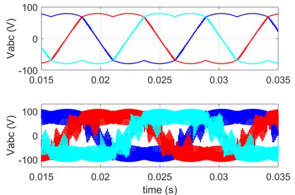
Fig. 5. OS-DB voltage references. Top panel: compensated OS-DB. Bottom Panel: uncompensated OS-DB.
