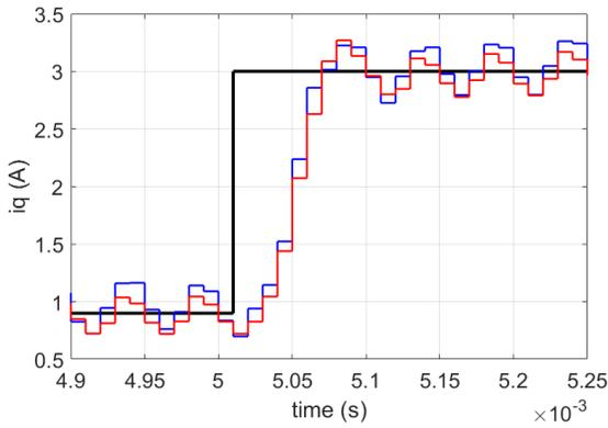
Fig. 12.  $i_q$  step from 0.9 to 3 A at  $\omega_m$  of  $130 \frac{rad}{s}$ . Reference current  $i_q$  (black line), FPGA DB  $i_q$  (blue line), OS-DB  $i_q$  (red line).
