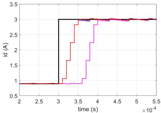
Fig. 4. System response to a reference  $i_d$  step from 0.9 to 3 A. reference current  $i_d$  (black line), DSP DB  $i_d$  (magenta line), FPGA DB  $i_d$  (blue line), OS-DB  $i_d$  (red line).
