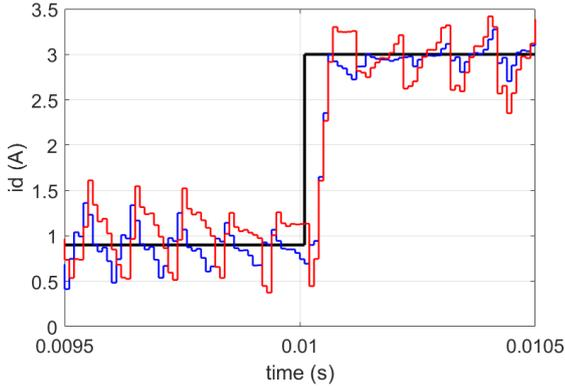
Fig. 11.  $i_d$  step from 0.9 to 3 A at  $\omega_m$  of  $150 \frac{rad}{s}$ . Reference current  $i_d$  (black line), FPGA DB  $i_d$  (blue line), OS-DB  $i_d$  (red line).
