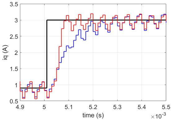
Fig. 16.  $i_q$  step from 0.9 to 3 A at  $\omega_m$  of  $100 \frac{rad}{s}$ . Reference current  $i_q$  (black line), FPGA DB  $i_q$  (blue line), OS-DB  $i_q$  (red line).
