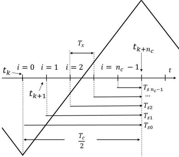
Fig. 1. Carrier and variable sample time for the OS-DB.
