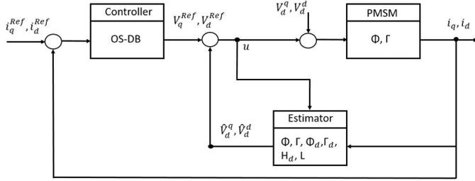
Fig. 3. Block scheme of the complete control structure.
