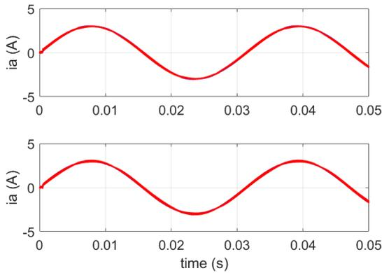
Fig. 8. OS-DB phase current steady state performances at  $\omega_m 50 \frac{rad}{s}$ . Top panel: 50%  $L_d$  increment. DB FPGA implemented  $i_a$  (blue line), OS-DB  $i_a$  (red line). Bottom Panel: 50%  $L_d$  reduction. DB FPGA implemented  $i_a$  (blue line), OS-DB  $i_a$  (red line).
