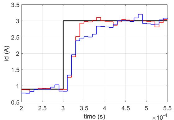
Fig. 6. OS-DB response to a reference  $i_d$  step from 0.9 to 3 A. Reference current  $i_d$  (black line), uncompensated OS-DB  $i_d$  (blue line), compensated OS-DB  $i_d$  (red line).
