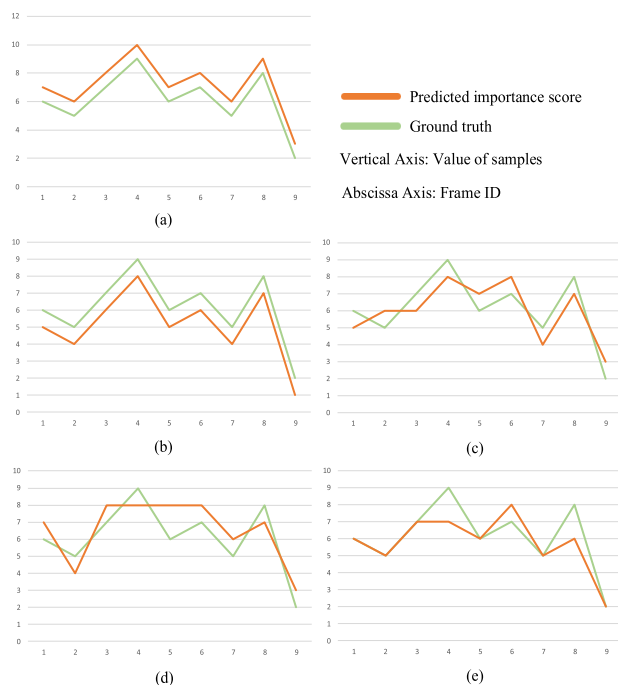
Fig. 2. Distributions of different predictions, where (a)–(e) have the same ground-truth sequences but different predicted importance score sequences. Although they have different distributions, they have the same mse (mse = 1.0). (a) Possible distribution 1. (b) Possible distribution 2. (c) Possible distribution 3. (d) Possible distribution 4. (e) Possible distribution 5.
