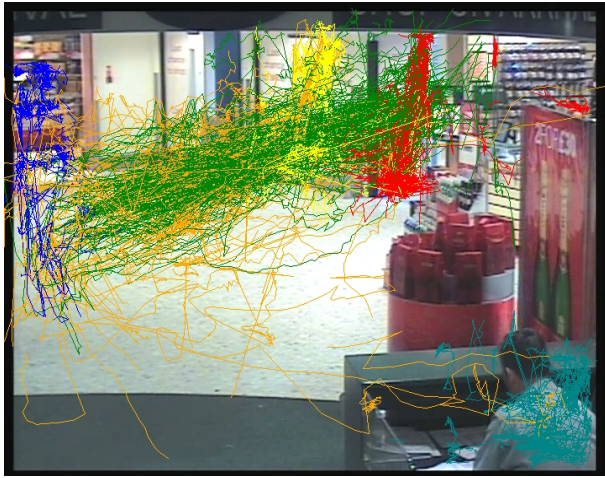
Fig. 6. Examples of trajectory clustering results obtained by EM algorithm on trajectories from the first camera.
