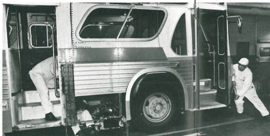
TIGHT FIT —The sections now have been joined but work to make the connection complete still has to be done, including rewiring of electric lines and other control systems. Later, 16 seats will be installed, providing 21 inches of seating space per passenger. Seats across back will be even wider.
