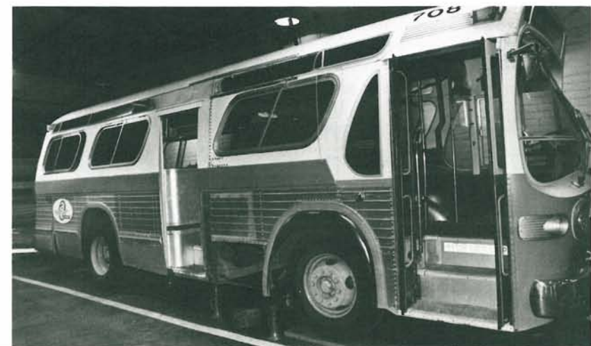
SURGERY COMPLETE —Back together again but more than five feet shorter, the bus is ready for final connections and repainting. The bus still has the same power plant, automatic heating and ventilation system, and the complete air ride originally in the bus but unavailable in smaller coaches.
