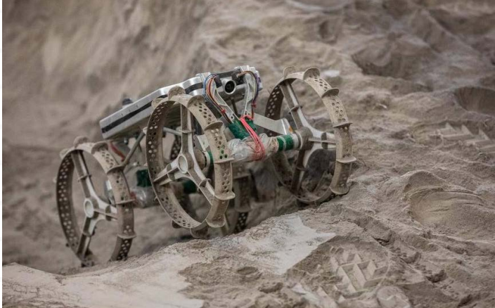
CubeRover mobility testing in regolith simulant.
