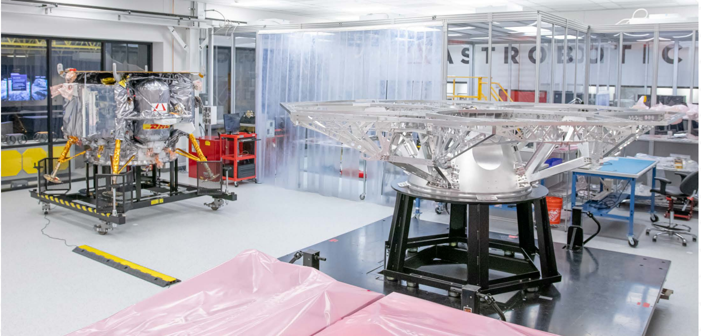
Astrobotic Headquarters contains two 100k (ISO Class 8) cleanrooms for integration activities.
