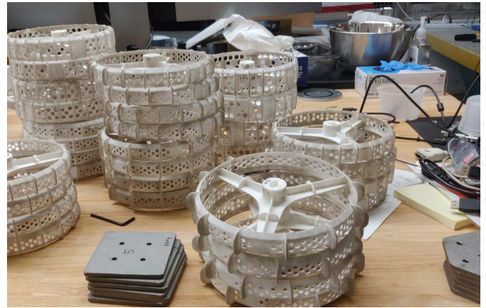
3D-printed CubeRover wheel prototypes.
