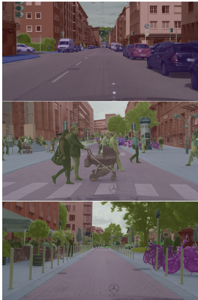
Figure 1. Example images (2 MP, color, HDR) with annotations from our dataset. The labels are encoded in different colors. Note that instances of traffic participants are annotated individually.
