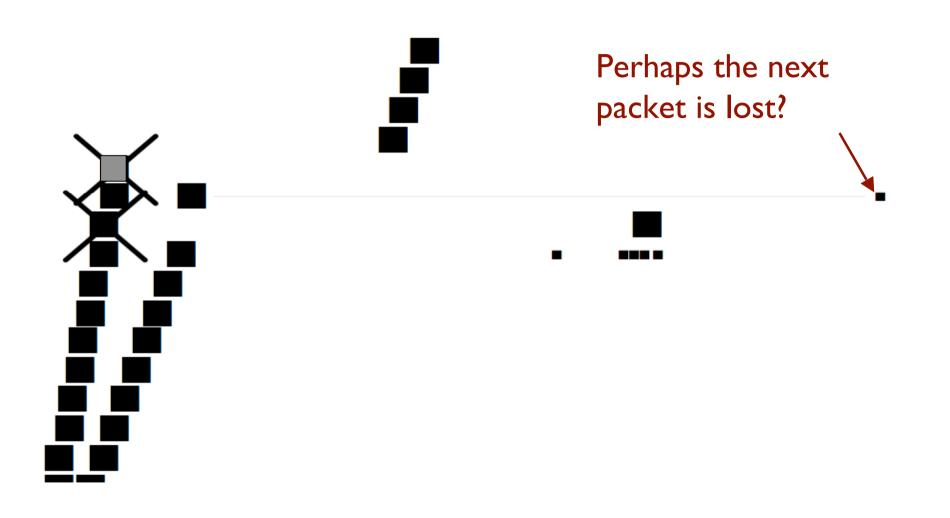
**3rd dup ack:** retransmit Ist unacked ssthresh = cwnd/2cwnd = cwnd/2 + 3remember highest
