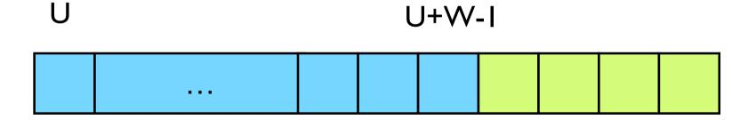
Between time t and t+RTT, the cwnd becomes W/2 + W-1. So we get to send W/2 new packets during the time. (Soon cwnd is going to become W/2 anyway..)
