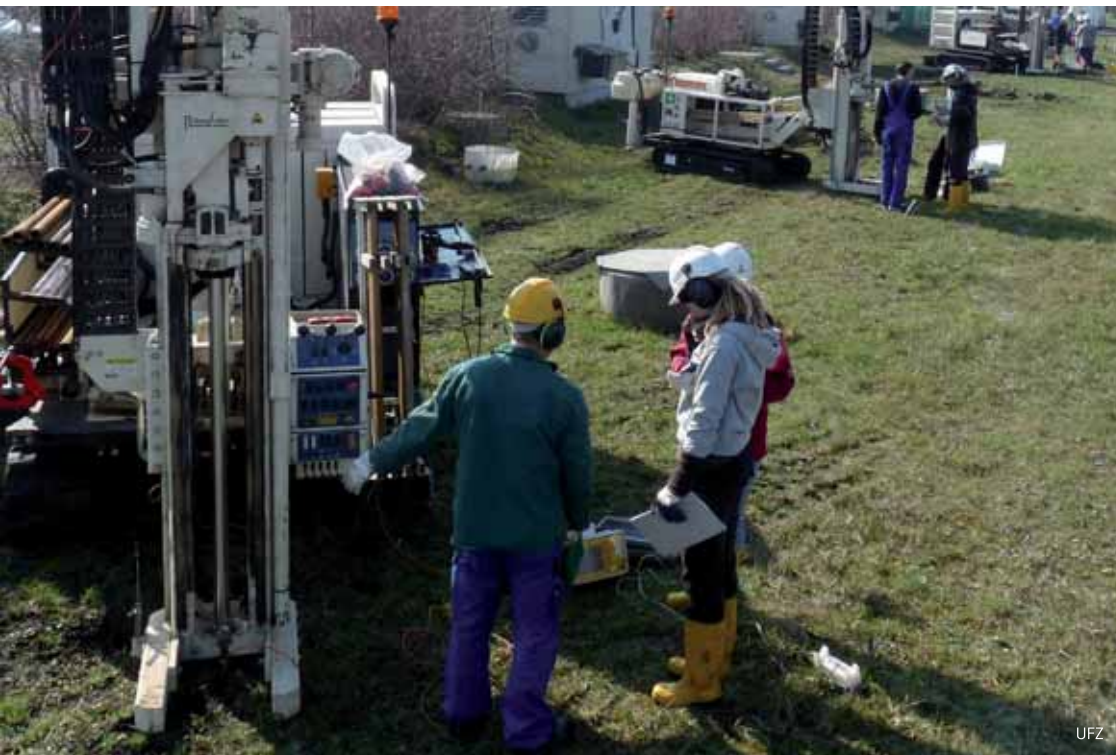
Application of direct push-technologies in the field for investigation of contaminated aquifers.
