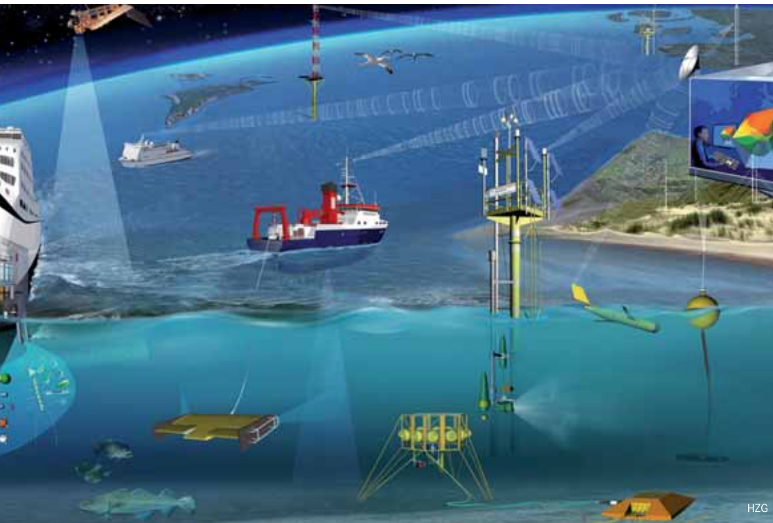
Sketch of observational platforms used for COSYNA, including satellites, hydrographic radar, fixed platforms, ferryboxes, underwater nodes and frames, wave buoys, gliders and research vessels.
