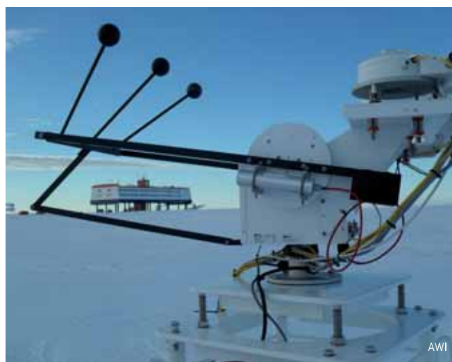
Antarctic base Neumayer III and instrumentation for measuring surface radiation balance.
