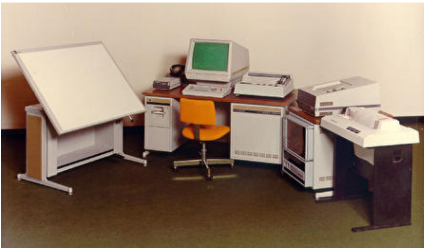
Fig. 28. The first “personal computer” that Cleve Moler ever used was the Tektronix 4081, which Argonne National Laboratory acquired in 1978. The machine was the size of a desk and consisted of a Tektronix graphics display attached to an Interdata 7/32, the first 32-bit minicomputer. There was only 64 kilobytes of memory—but there was a Fortran compiler, and so, by using memory overlays, it was possible to run MATLAB. (Source: Ned Thanhouser.)
