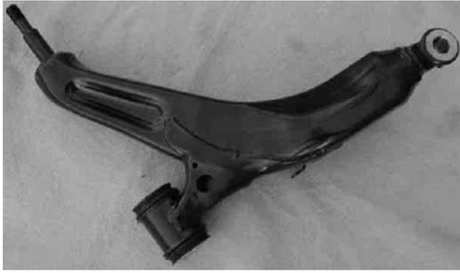
Photo 2 Lower arm to which 780 MPa grade developed steel tube is applied
