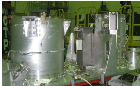
Figure 17: The first P-POD Mark II with MAST inside mounted to the Space Head Module. The other two P-PODs will be mounted on the same mounting plate.
