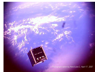
Figure 21: CP4 in space. This picture was taken by AeroCube-2 (Section 3.6.2) a few minutes after ejection from the P-POD.
