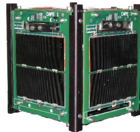
Figure 23: CAPE1. The turnstile antenna doors are visible above the solar cells.
