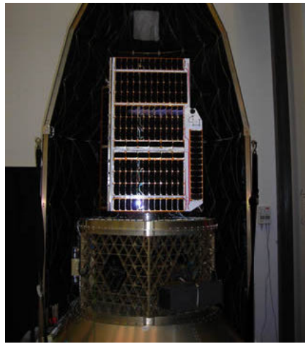
Figure 33: Upper stage of the Falcon 1 launch vehicle. The P-POD Mark III is mounted in the lower right.
