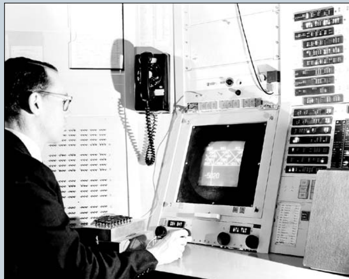
Ivan Sutherland is shown working with Sketchpad. The lightpen, shown below, and the keyboard function control are the precursors for the mouse and right and left mouse-clicks prevalent today.
