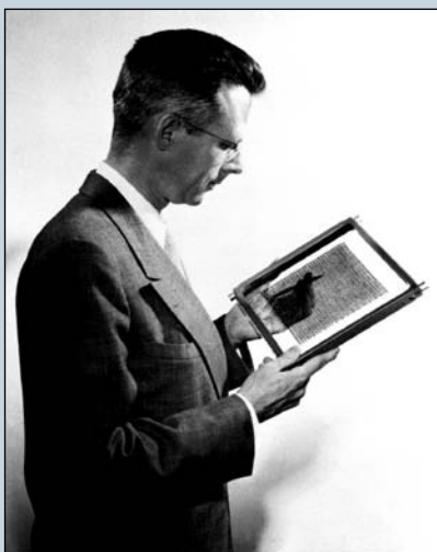
Jay Forrester is holding a magnetic-core memory .
