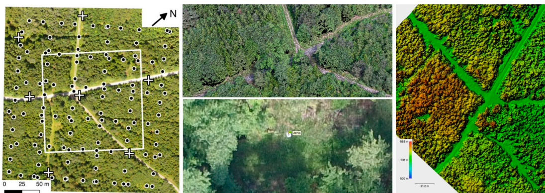
Figure 1. Orthomosaic from 27 May 2017 of the study area in Hungerbrunnen, Rottenburg Municipal Forest, centered at latitude/longitude 48.44923° / 8.96557°. Overlaid are camera positions of the flight mission on 8 July 2017 (black dots), the positions of the ground control plates (white crosses) and the center square of the study area used for tree height growth measurements (white square). Upper middle: 3D dense point cloud of the center of the study area. Lower middle: UAV aerial photograph of the north-western ground control plate. Right: subset of the digital surface model of the data acquisition on 27 May.
