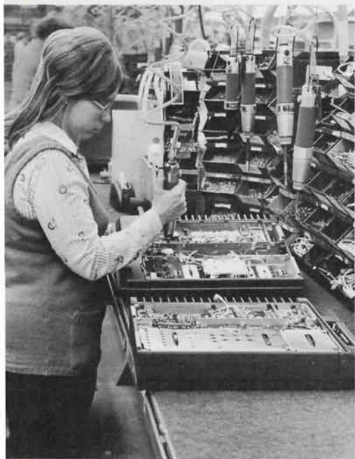
900 MHz radios in production at the Schauburg facility.
