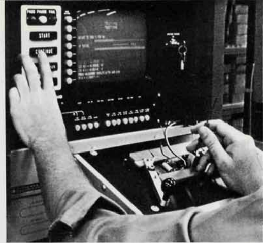
An employee in the division's Seguin, Texas facility aligns a radio panel using sophisticated automatic test equipment installed during 1975.
