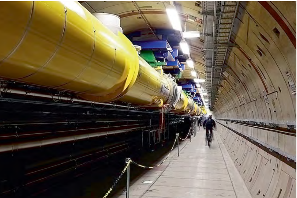
A racetrack for electrons: In the XFEL free-electron laser, particles whiz through a 3.4-kilometer-long tunnel between the DESY research center in Hamburg-Bahrenfeld and Schenefeld (top), producing X-ray flashes in the process. Employees travel through the X-ray laser tunnel on bicycles (bottom).
