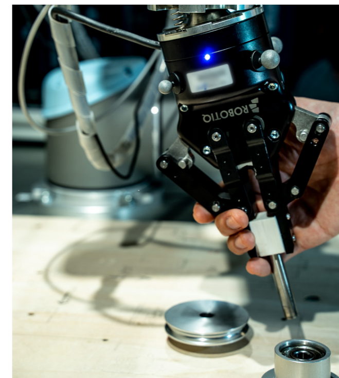
▲ Two examples of AI robots that can assist humans with tasks. The top one can grind materials in a mortar, while the bottom one can perform a peg-in-hole task.
