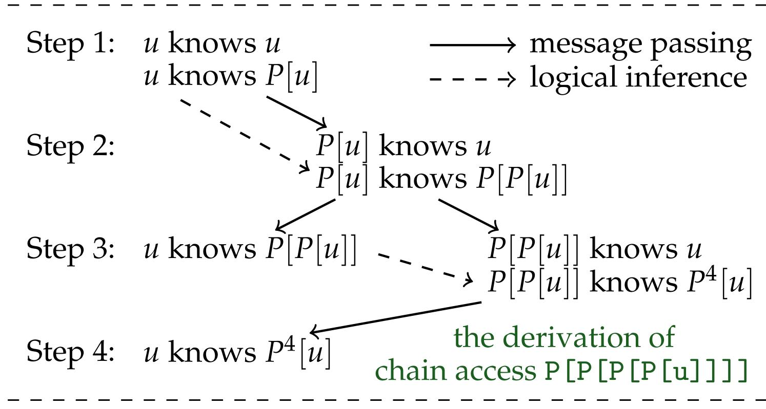
A backtracking algorithm with memoization for finding a solution with minimum number of steps Application: the pointer-jumping technique (a useful graph transformation used in S-V, MSF and so on)
