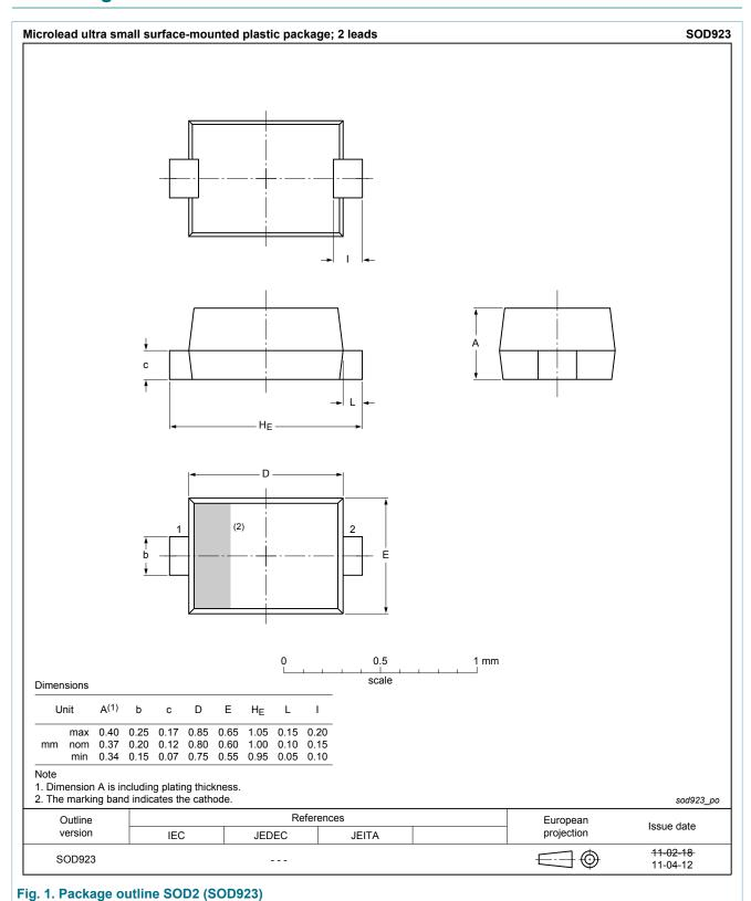
Microlead ultra small surface-mounted plastic package; 2 leads
