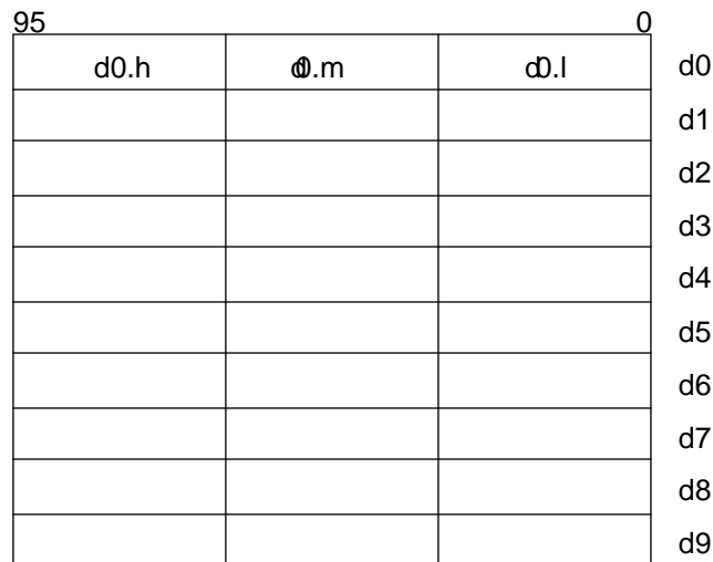
Figure C-9. The Data ALU's Register File
