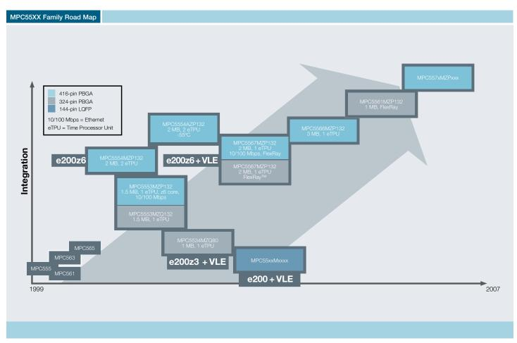
The MPC5567 combines the high performance characteristics of the e200z6 core architecture with high-level module functions, including FlexRay<sup>™</sup> technology, 10/100 Ethernet and enhanced Time Processor Unit (eTPU). The MPC5567 is particularly well suited for next-generation automotive applications because the FlexRay network will play a significant role in advanced chassis applications, such as stability control and brake-by-wire and steer-by-wire systems.
