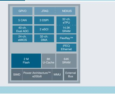
With the combined capabilities of FlexRay technology and Ethernet, along with five Controller Area Network (CAN) modules, the MPC5567 helps developers control costs when designing increasingly complex applications in automotive and industrial systems, such as:
