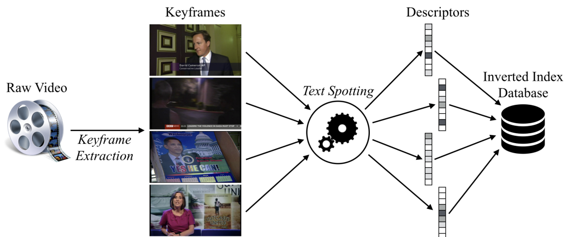
Figure 8.2: The processing pipeline for the video retrieval application. First, keyframes are extracted from the raw video file. Each of the keyframes are processed by the text spotting system of Chapter 5, producing per-image descriptors, encoding the text contained within the keyframe images. These descriptors are loaded in to an in-memory database with an inverted index for fast retrieval at query time.
