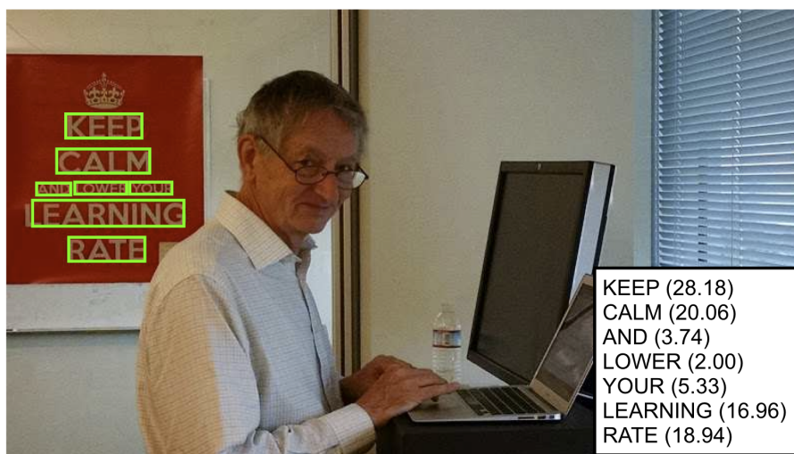
Figure 9.1: An example text spotting result using the pipeline of Chapter 5. The bounding boxes of each word found are shown in green, with the recognised words given in typographical layout order together with the score assigned by the pipeline in brackets.
