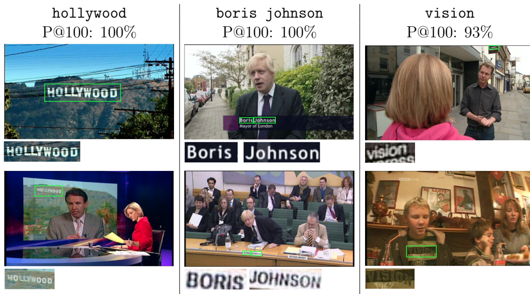
Figure 8.4: The top two retrieval results for three queries on our BBC News dataset – hollywood , boris johnson , and vision . The frames and associated videos are retrieved from 5k hours of BBC video. We give the precision at 100 (P@100) for these queries, equivalent to the first page of results of our web application.
