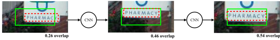
Figure 5.5: An example of the improvement in localisation of the word detection pharmacy through multiple rounds of recurrent regression.
