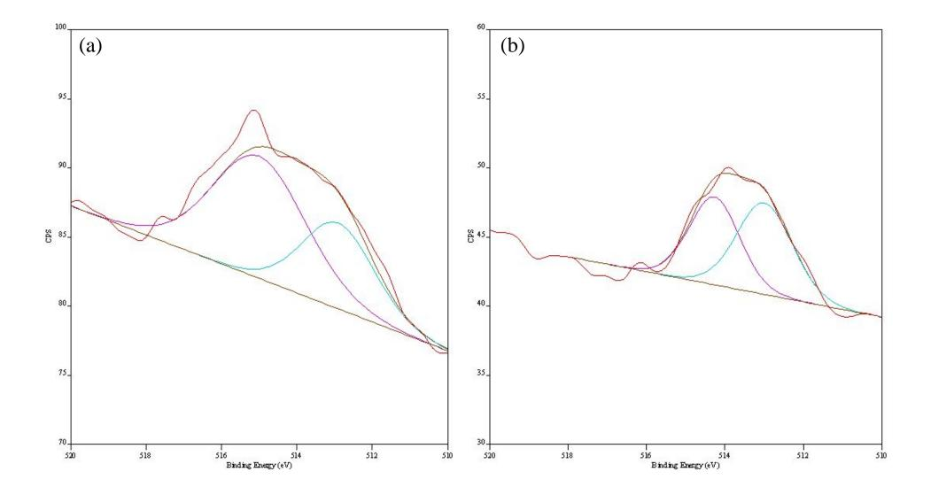
**Figure 2** –  $V2p^{3/2}$  region in the XPS spectra of phenol/formaldehyde resin after gas phase deposition of  $VOCl_3$  (a) before and (b) after argon bombardment. The ratio 4+:5+ increases from 35:65 to 47:53 after sputtering.
