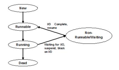
The following diagram shows the complete life cycle of a thread:
